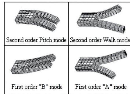
Fig. 2 Vibration modes of quartz tuning fork
