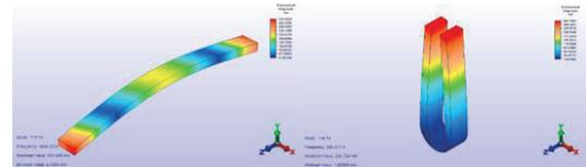
Fig. 1 The first-order vibration modes of free-free beam and U-Shape structure.
