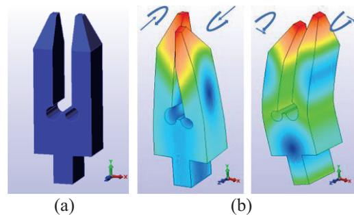
Fig. 3 (a) Original vibrator. (b) Schematic illustration of fundamental operation principle of the two vibration modes of quartz tuning fork
