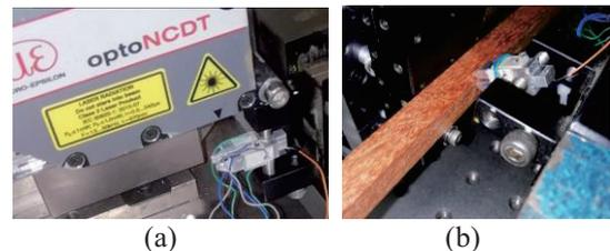
Fig. 4 (a) Photograph of the prototype piezoelectric linear motor and setup for the displacement measurement. (b) the performance test devices
