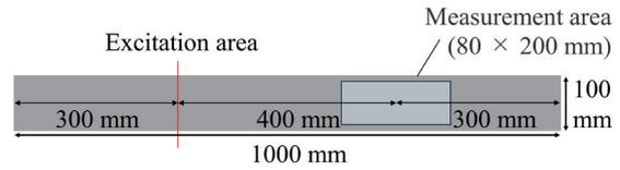
Fig. 3 Schematic view of sample and measurement area
