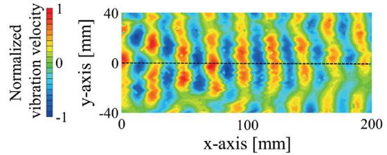
Fig. 4 Instantaneous vibration velocity distribution in measurement area
