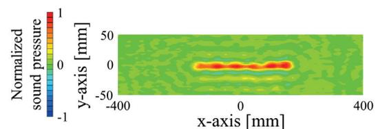
Fig. 2 Sound pressure distribution around open end of acoustic waveguide
