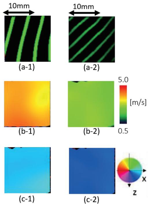
Fig.4 Shear wave maps measured in the chicken phantom. (a) Shear wave propagation map, (b) velocity map and (c) direction map. (a-1)-(c-1) and (a-2)-(c-2) were observed by x- and z-direction enhancement, respectively.
