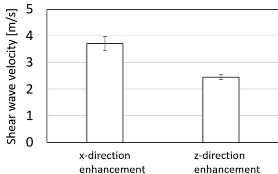
Fig. 5 Shear wave velocity obtained from x- and z-directional enhanced images
