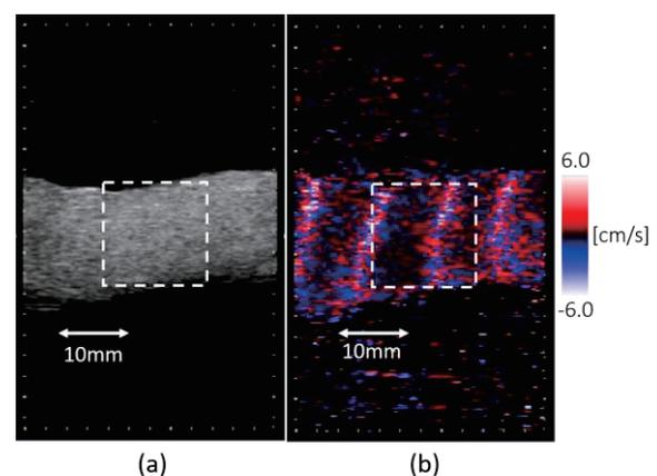
Fig. 2 Chicken phantom image. (a) B-mode image, (b) CFI
