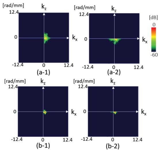
Fig.3 Wavenumber spectrum separated in x-direction and z-direction (a-1),(a-2) and applied Wiener filter (b-1),(b-2)
