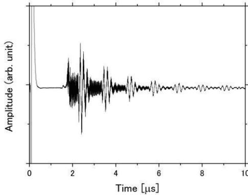
**Fig. 2** Ultrasonic response at 700°C in the 1st cycle of CBTa/BiT sample.
