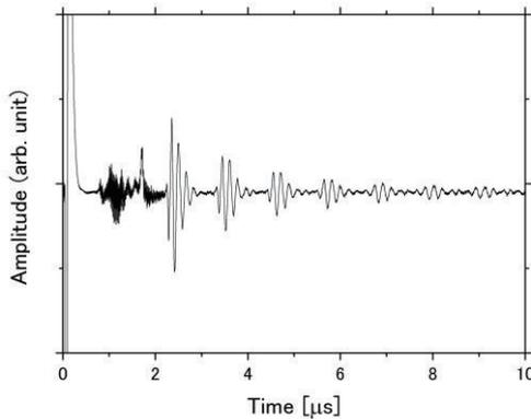
**Fig. 3** Ultrasonic response at 700°C in the 3rd cycle of CBTa/BiT sample.
