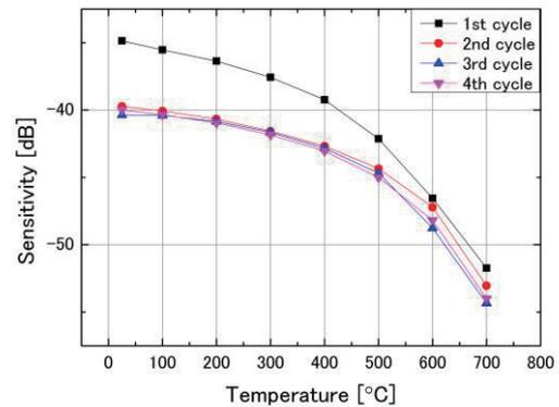
**Fig. 4** Sensitivity of CBTa/BiT sample at various temperatures during thermal cycle test.
