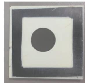
Fig. 1 Optical image of CBTa/BiT film on 3mm thick titanium substrate.
