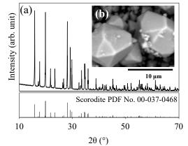
Fig. 1 (a) XRD pattern and (b) SEM image of sample synthesized using ultrasound irradiation.
