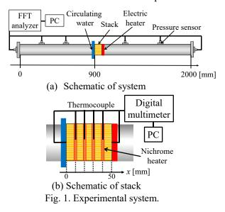
heat equilibrium for each input electric power  $W_1$  of the internal heater increases as 15, 40 and 60 W is measured after each equilibrium is attained in about 20 min. Furthermore, measuring the sound pressure and the resonance frequency in the tube with a crystal type pressure sensor (PCB Inc.), the work flow distribution is estimated from these data[5].
