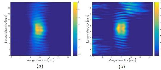
Figure2: B-mode image of the SA-SCM using (a) DAS and (b) F-DMAS.
