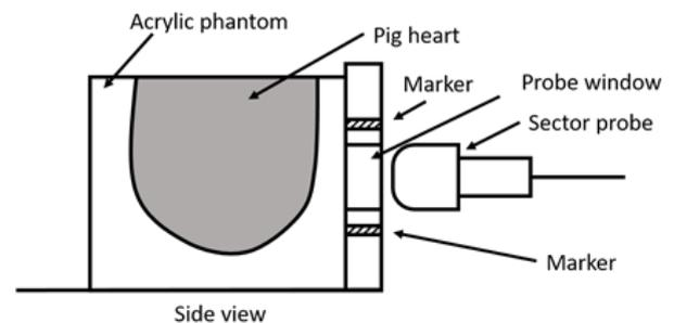
Fig. 1 Experimental system for US image.
