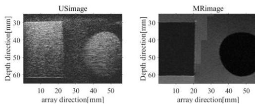
Fig.3 Ultrasonic image (left) and MR image (right) of the phantom.
