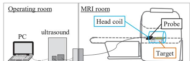
Fig.2 Experimental system of US and MR simultaneous multimodality imaging.
