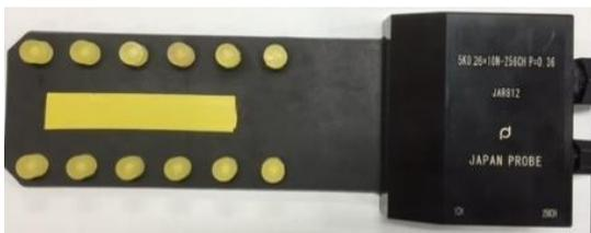
Fig.1 The prototype array probe attached with MR visible fiducial markers. The specification of the probe is listed in Table 1.
