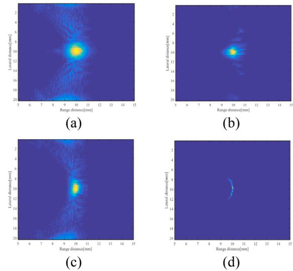
Fig. 2. B-mode images of experiment results: (a) averaged SA; (b) SA-SCM; (c) averaged SCM-weighted SA; (d) SCM-weighted SA-SCM.
