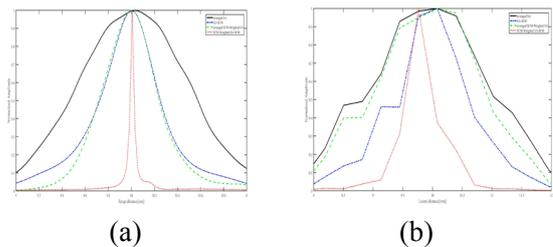
Fig. 3. Comparison of normalized cross-sectional profile: (a) range profile; (b) lateral profile.
