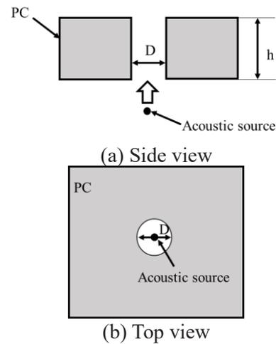
Fig. 1 Illustrations of the relationship between cylindrical waveguide and acoustic source in (a) side view, and in (b) top view.
