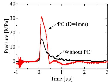
Fig. 2 Typical pressure waveform. The red and black lines indicate the waveform through cylindrical waveguide (a diameter  $D$  of 4 mm) and without a PC plate, respectively.
