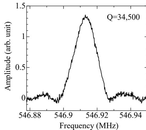
Fig. 3 Resonance spectrum of wireless MEMS QCM chip in the atmosphere.
