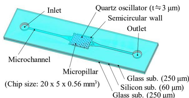
Fig. 1 Schematic of wireless MEMS QCM chip.
