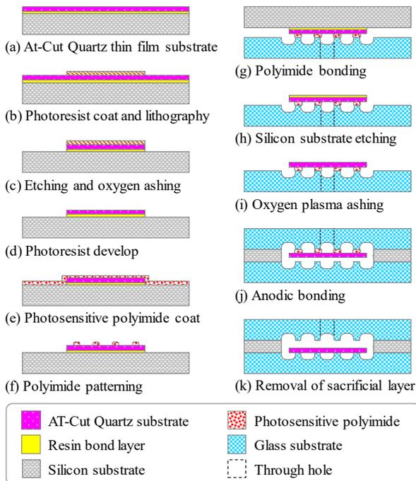
Fig. 2 Wafer-level package process steps using polyimide sacrificial layer.
