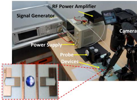
Fig. 2 The experimental setup and a realized device.
