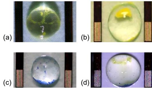
Fig. 4 SAW manipulation results. (a)  $2\text{-}\mu\text{m}$  particles, without PCs. (b)  $2\text{-}\mu\text{m}$  particles, with PCs. (c)  $20\text{-}\mu\text{m}$  particles, with PCs. (d) Mix of  $2\text{-}$  and  $20\text{-}\mu\text{m}$  particles, with PCs.
