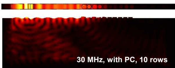
Fig. 3 Calculated results of 30-MHz SAW stopped by the PCs.
