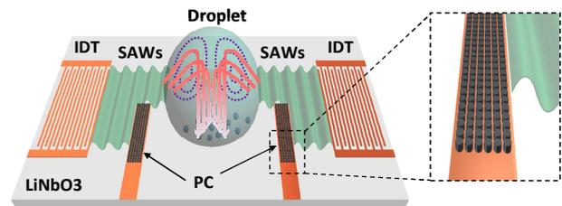
Fig. 1 Schematic of the SAW based acoustofluidic platform with PCs for manipulating microparticles inside a sessile droplet.
