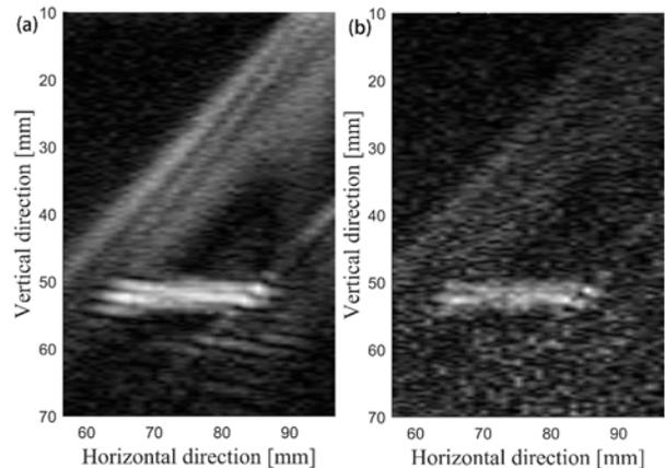
Figure.4 (a) the image of Barker code excitation (b) the image of single pulse excitation
