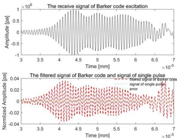
Figure.3 (a) acquisition of Barker code excitation (b) contrast of filtered signal
