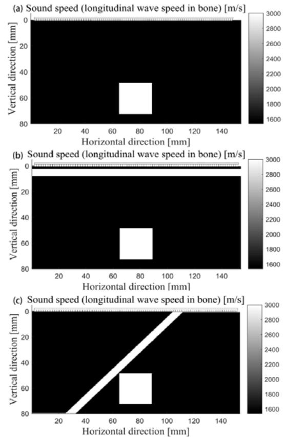
Figure.1 the geometric settings (a) without skull bone (b) horizontally arranged (c) with an angle of  $\pi/4$
