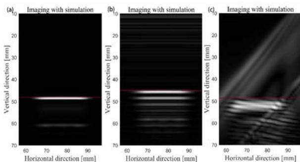
Figure.2 the images (a) without skull bone (b) horizontally arranged (c) with an angle of  $\pi/4$
