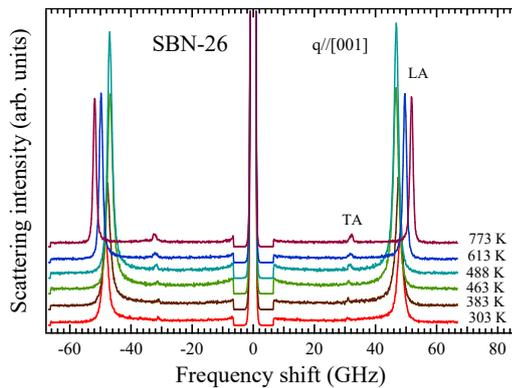
Fig. 3 Brillouin scattering spectra of the *c*-plate of a SBN26 crystal with very weak RFs.
