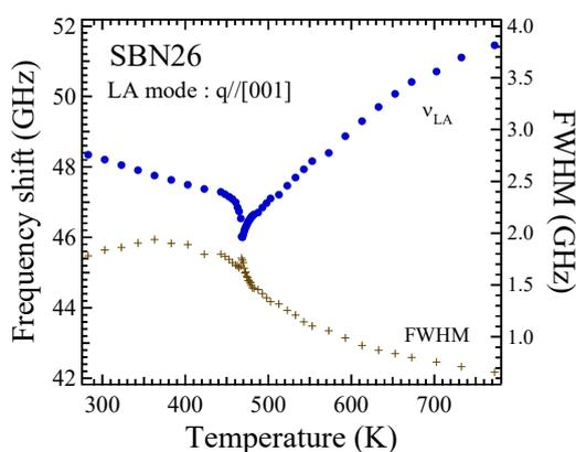
Fig. 4 Temperature dependence of the frequency of the LA mode along the *c*-axis of a SBN26 crystal.
