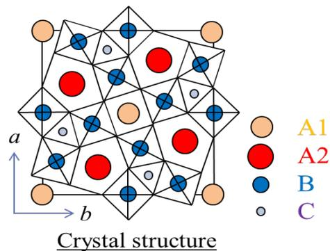
Fig. 1 Crystal structure of TTB ferroelectrics along the  $c$ -axis.
