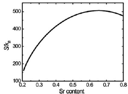
Fig. 2 Lattice entropy of strontium barium niobate with TTB structure [2].
