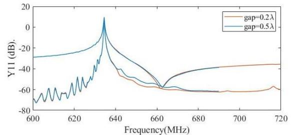
Fig. 3 Simulated Y11 curves of SAW resonator
