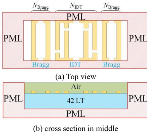
Fig.2 Schematic of the final 3D FEM model
