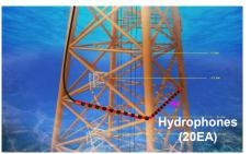
Fig. 1 Concept diagram of hydrophone installation
