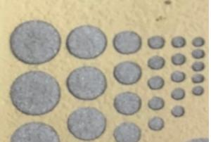
Fig.1 Picture of fabricated top electrodes on sol-gel composite piezoelectric sensor.
