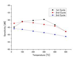
Fig.4 Sensitivity of BiT/TiO<sub>2</sub> sample at various temperatures during thermal cycle test.
