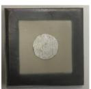
Fig.1 50 $\mu$ m thick BiT/TiO<sub>2</sub> film with silver top electrode on 3mm thick titanium substrate.
