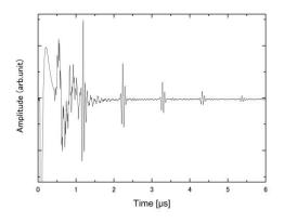
Fig.2 Ultrasonic response at 500°C in the  $3^{rd}$  cycle of BiT/TiO<sub>2</sub> sample fired at 400°C.
