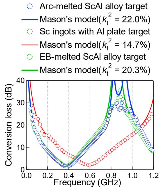
Figure 2. Experimental and theoretical conversion loss curves of ScAlN films made by Arc-melted ScAl alloy target, Sc ingots with pure Al plate target, and electron-beam melted ScAl alloy target. The theoretical curves were simulated by Mason's equivalent circuit model including the electrode layers.
