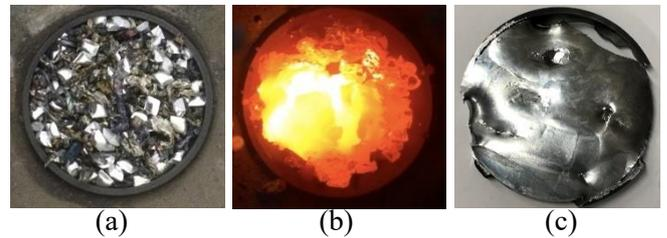
Figure 1. Typical images of (a) Al and Sc ingots placed on a carbon plate, (b) electron-beam melted ingots and (c) resulting lab-made ScAl alloy target (the third target).
