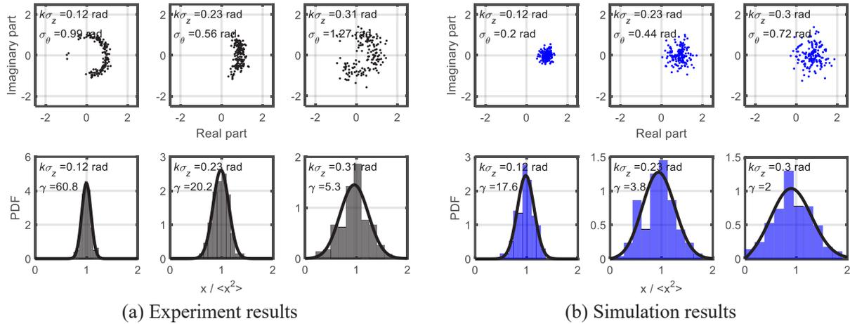
Fig.5 150 signals on complex plane and PDF, fitting result to the Rice distribution (12.5 kHz)
