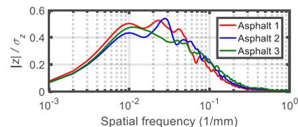
Fig.3 Spatial frequency spectra in  $x$  directions on the road surface
