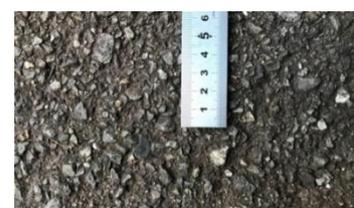
(c) Asphalt 3 ( $\sigma_z = 0.52$  mm)
