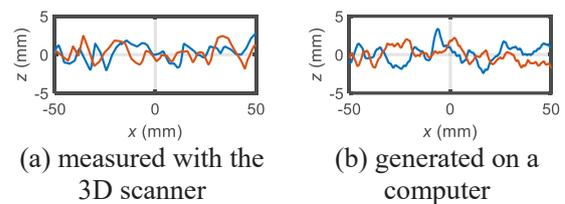
Fig.2 Cross-section shape of road surfaces ( $\sigma_z = 1.0$  mm)
