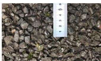
(b) Asphalt 2 ( $\sigma_z = 1.0$  mm)
