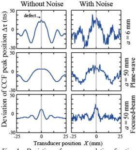
Fig. 4 Deviation of cross correlation function peak position  $\Delta \tau$  of each transmitter arrays and transmitting wave shapes.
