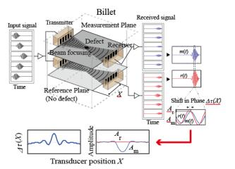
Fig. 1 Outline of defect detection inside billet by transmission method using phased array technique.
