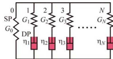
Fig. 2  $N$ -element generalized Maxwell solid model. SP and DP represent a linear spring (spring constant  $G$ ) and a dash pot. (viscosity  $\eta$ ), respectively. The relaxation time is expressed by  $\tau_G^{(j)} = \eta_j / G_j$  ( $j=1,2,3,\dots,N$ ).
