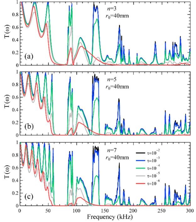
Fig. 3 Transmission rate vs frequency for (a)  $n=3$ , (b)  $n=5$ , and (c)  $n=7$ , respectively. The incident wave is longitudinal one. The colorful solid lines denote the differences of the relaxation time.
