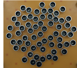
Fig. 1 Parametric loudspeaker with random element arrangement.
