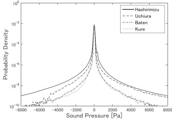
Fig. 1 Amplitude histograms of ambient noise observed at several coastal waters in Japan
