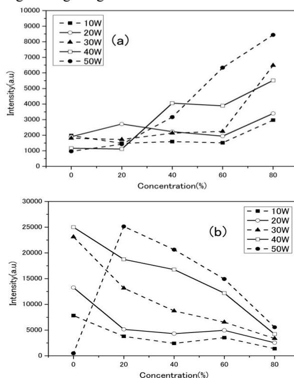
Fig.1 Viscosity dependences of SL intensity at 50 kHz (a), 150 kHz (b) in aqueous solutions of glycerol for various input powers.
