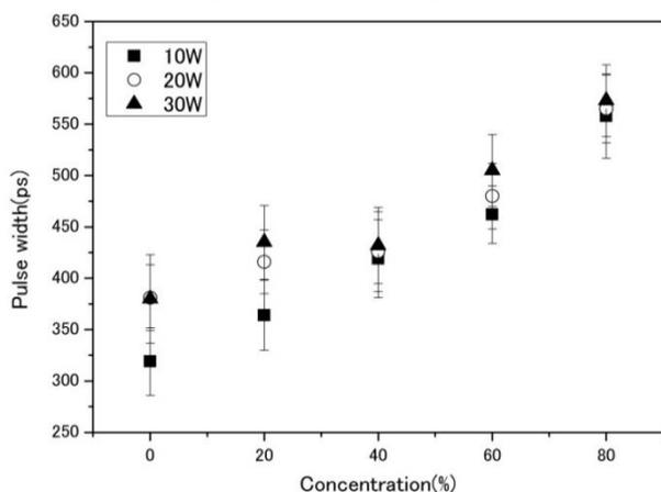
Fig.3 SL pulse width observed with different glycerol concentrations at 50 kHz.
