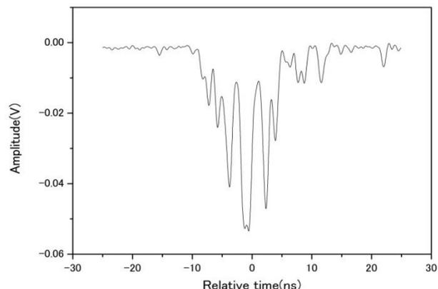
Fig.4 The multiple-peak pulse from NaCl glycerol solutions saturated with krypton at 28 kHz.
