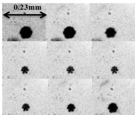
Fig.2 High speed images of bubble dynamics taken at the speed of 500kfps at 50 kHz in 80% glycerol solutions.
