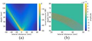
Fig. 3 (a) Sound pressure field and (b) grating lobe component obtained with conventional waveform (rectangular apodization).
