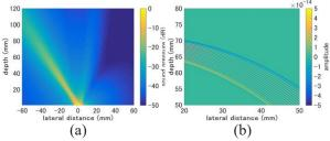
Fig. 5 (a) Sound pressure field and (b) Grating lobe component obtained with proposed waveform (Tukey apodization).
