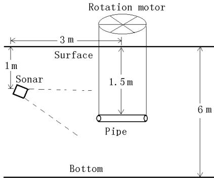
Fig. 3 Experiment setup
