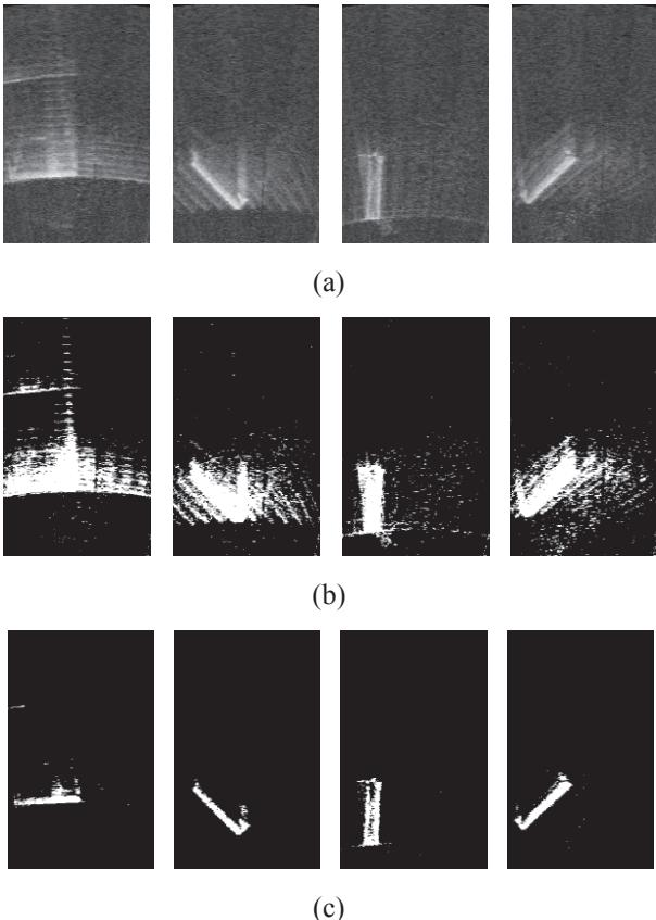
Fig. 4 Segmentation results (from the left to the right: 0 degree, 45 degrees, 90 degrees, and 135 degrees): (a) original sonar images; (b) Otsu; (c) the proposed method.
