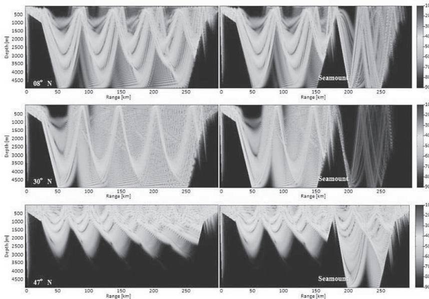
Fig.3 Calculation results of the sound wave propagation of distance 300 km by PE method. (Left: flat seabed, Right: seamount (500 m) at a distance of 180km)
