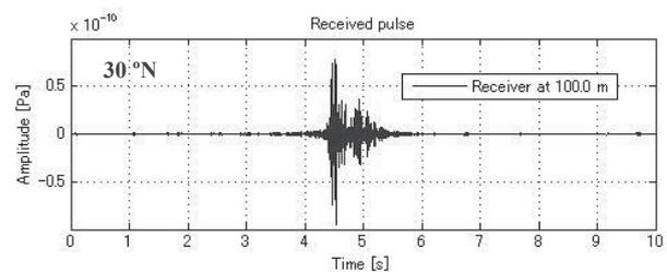
Fig.5 The received wave pulse shape (wave receiving depth 100m)
