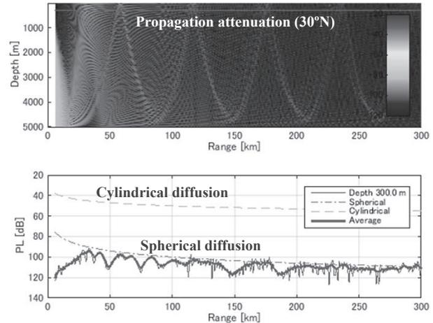
Fig.4 Propagation attenuation characteristics
