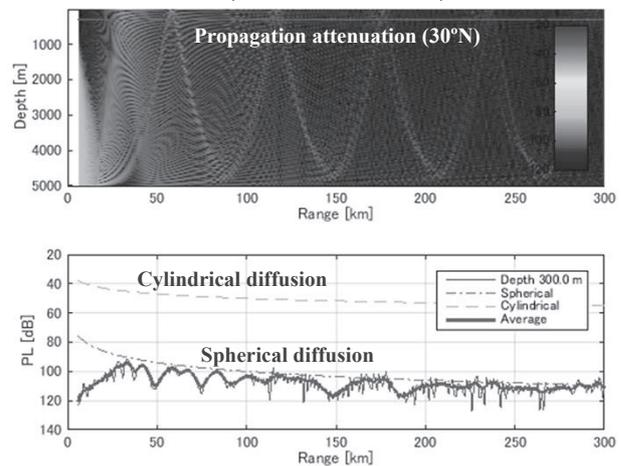
Fig.4 Propagation attenuation characteristics
