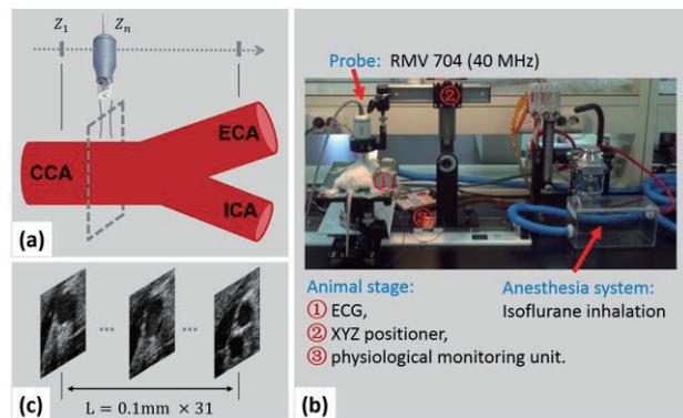
Fig. 1. A protocol of ultrasound image acquisition with setting. (a) Mechanical linear scanning from common carotid to external and internal carotid artery. (b) Experiment setting. (c) The portion slices of acquired 3-D data set
