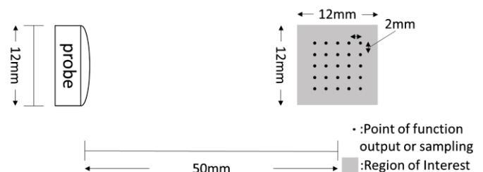
**Fig. 1** Imaging cross-section spanned by range and elevation directions.
