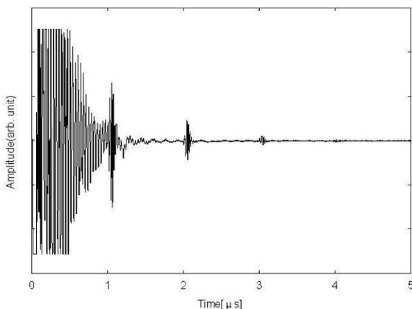
Fig.3: Ultrasonic response of PZT-2/PZT sample onto  $\sim 3\text{mm}$  titanium substrate
