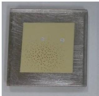
Fig.2: PZT-2/PZT sample onto a titanium substrate sintered by a domestic microwave oven.
