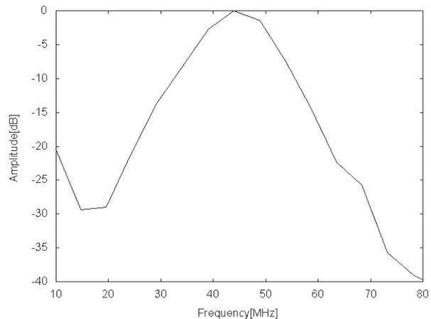
Fig.4: Frequency characteristic of PZT-2/PZT sample onto titanium substrate
