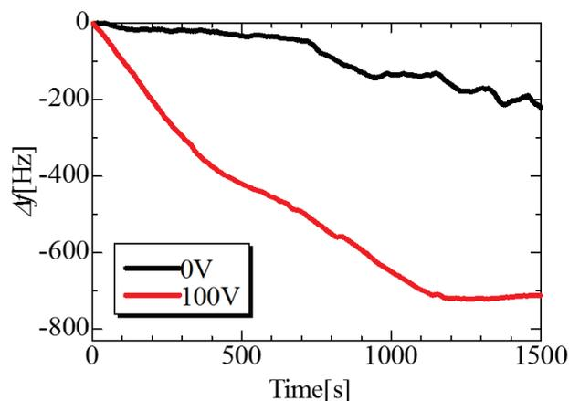
Fig. 2 Comparison lines about frequency shifts by immobilizing aptamers on the sensor chip. Black line shows the result of not applying electrostatic pressure and Red line shows that of applying electrostatic pressure.
