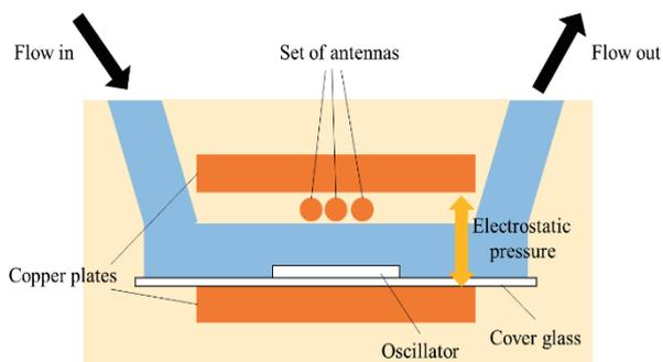
Fig. 1 Experimental Schematic of contactlessly measuring the resonance frequency of the quartz oscillator with applying the electrostatic pressure contractually by the copper plates.
