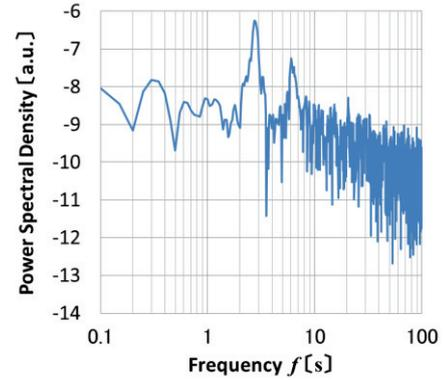
**Fig. 4.** Power spectral density of the variation of the angle  $\theta = \angle P_1P_2P_3$ .
