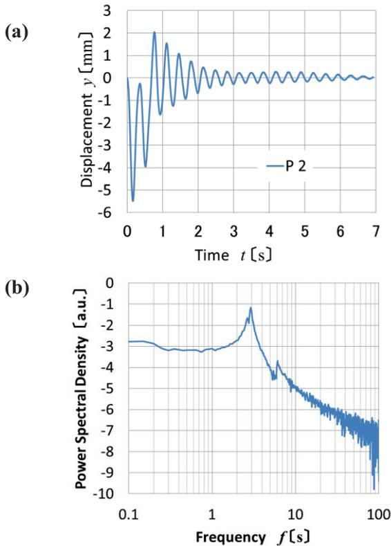
**Fig. 3.** A typical result of the vibration measurement of a leaf. (a)Vibration displacement of point P2, (b) its power spectral density.
