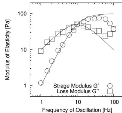
Fig. 3 Dynamic viscoelasticity of wormlike micellar solution. The solid line shows single viscoelastic relaxation.
