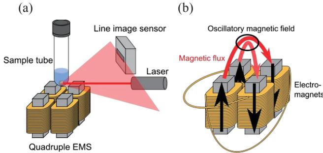
Fig. 1 Schematic view of Quadruple EMS system. (a) Entire view of this system. (b) Generation of oscillatory magnetic field by electromagnets.
