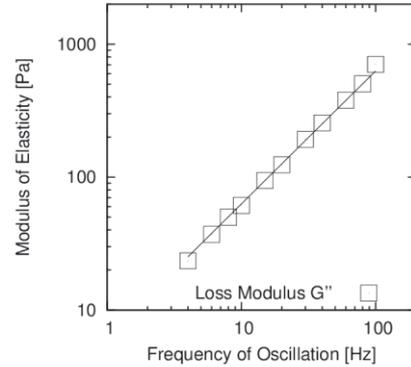
Fig. 2 Dynamic modulus of Newtonian sample and determination of apparatus constant. The loss modulus is proportional to the frequency. The solid line is given by  $G'' = \eta\omega$ .
