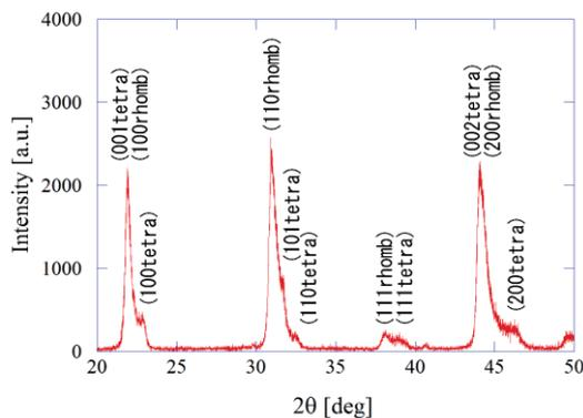
Fig. 4 XRD pattern of the PZT film deposited with condition III
