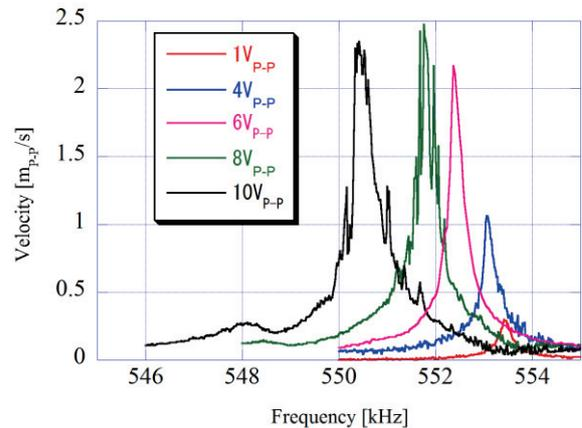
Fig. 5 Vibration velocity of the transducer at the tip
