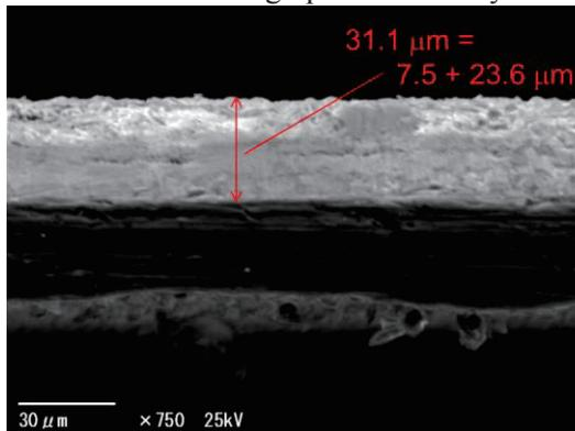
Fig. 3 Cross-sectional SEM image of the PZT film deposited with condition III
