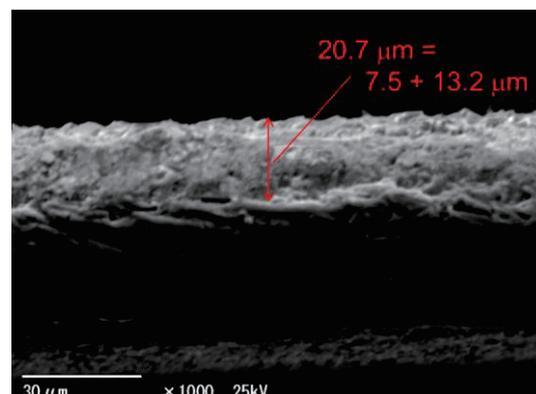
**Fig. 1** Cross-sectional SEM image of PZT film deposited with condition II
