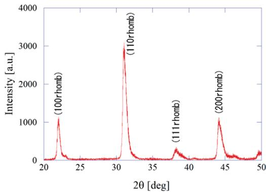
Fig. 2 XRD pattern of the PZT film deposited with condition II
