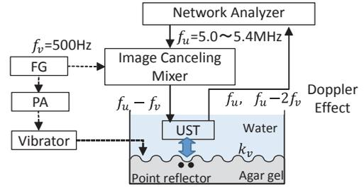
Fig. 1 SFCW vibro-Doppler measurement system
