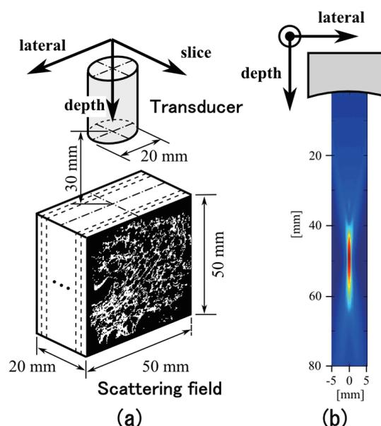
Fig. 1 (a) Schematic image of the simulation setup (b) Emitted sound field with used transducer for simulation
