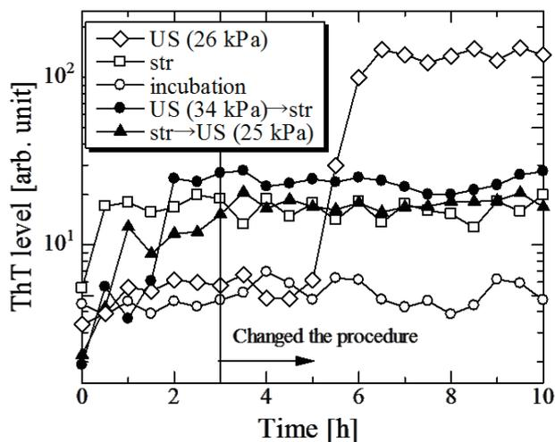
Fig. 1 Time courses of ThT level caused by ultrasonic irradiation (US), stirring (str), and incubation procedures.
