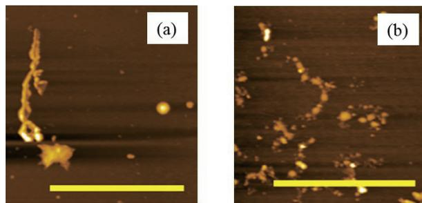
Fig. 2 AFM images of aggregates formed with (a) ultrasonic irradiation and (b) stirring procedure. Scale bars indicate 5  $\mu$ m.
