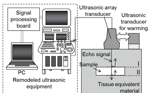
Fig.1 Ultrasonic velocity-change imaging system for quantitative assessment of fat content
