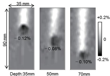
Fig.5 Ultrasonic velocity-change images of tissue phantom including fat areas (fat content of 30%) located at 30mm, 45mm and 70mm in depth from the surface, individually..
