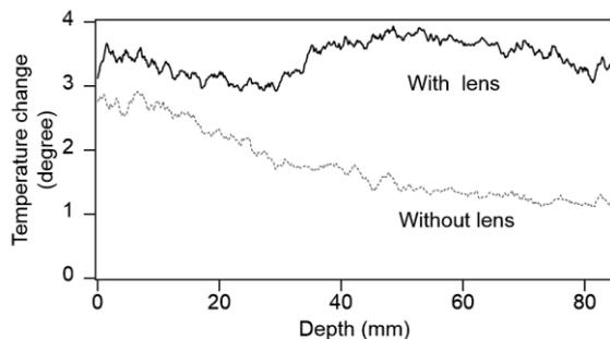
Fig.3 Profiles of temperature change in the phantom along the dotted lines in Fig.2(b)
