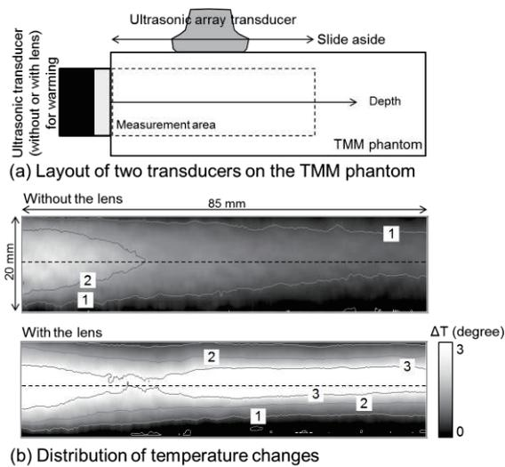
Fig.2 Temperature change distribution obtained by ultrasonic warming
