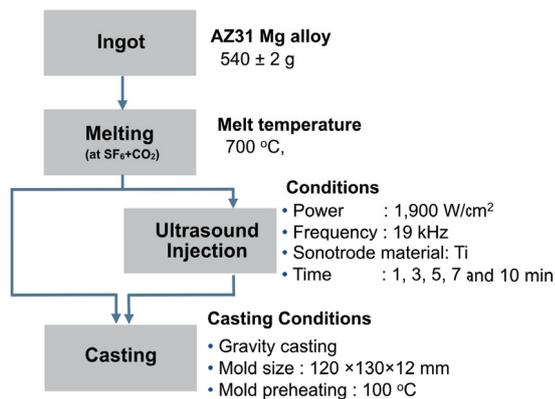
Fig. 1. Experimental procedure
