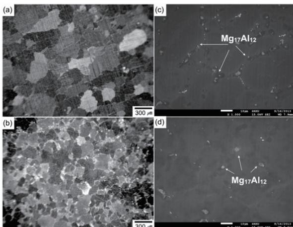
Fig. 2. Macro((a) and (b)) and grain boundary ((c) and (d)) structure of AZ31 alloy cast without ((a) and (c)) and with NEUMT((b) and (d))
