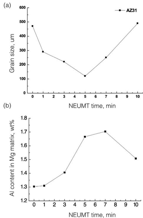
Fig. 3. (a) Grain size and (b) Al content in matrix of AZ31 alloy with increasing NEUMT time
