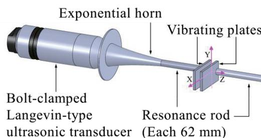
Fig. 1 Schematic diagram of the ultrasonic source.
