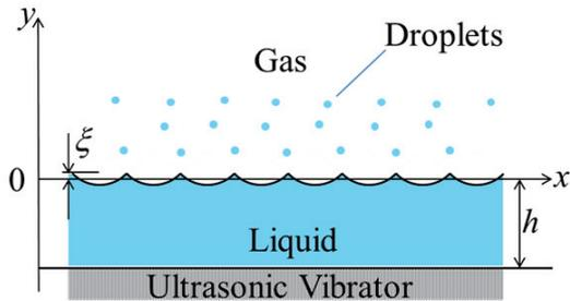
Fig. 1 Theoretical model of ultrasonic nebulizing.
