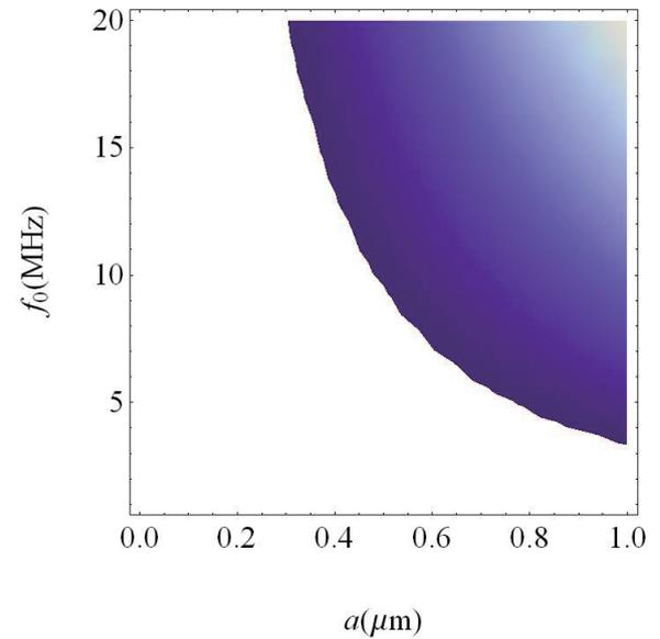
Fig. 3 Ultrasonic atomization condition for water.
