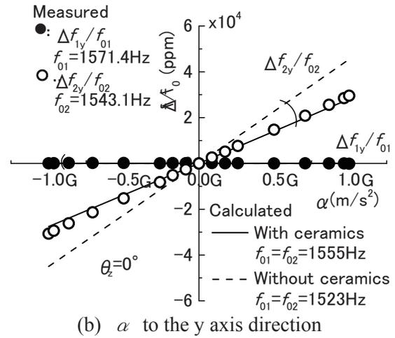
Fig. 6 Characteristics of sensor of trial production.
