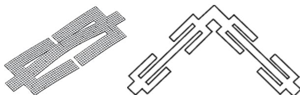
(a) Bending vibrator (b) Right-angled vibrator
