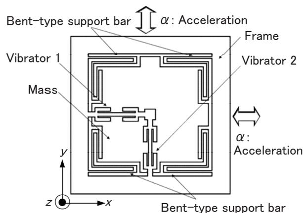
Fig. 2 Structure of two-axis acceleration sensor.
