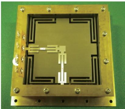
Fig. 5 Two-axis sensor of trial production.
