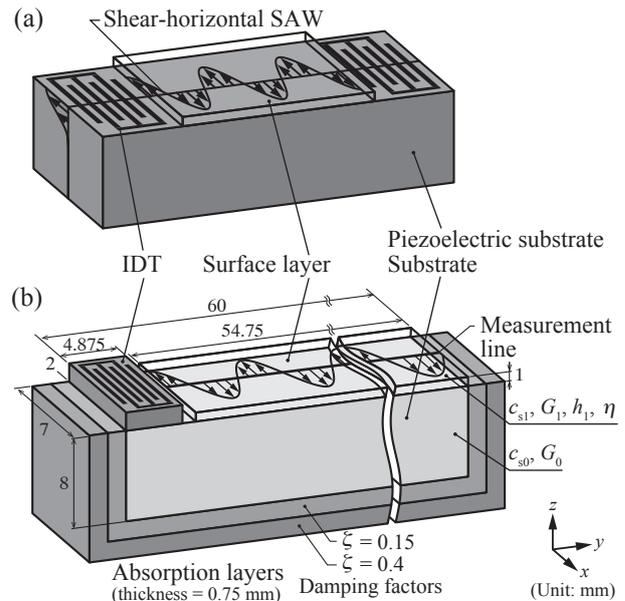
**Fig. 1** Comparison between (a) previous (using shear-horizontal SAW) and (b) proposed method (using Love-type wave) for viscoelasticity evaluation. The (b) also shows as simulation model of Love-type wave propagation for finite element method.
