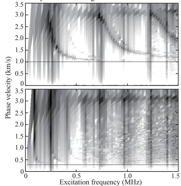
**Fig. 3** Dispersion curves of Love-type wave phase velocity when (a)  $G' = 1.185 \times 10^9$  Pa and (b)  $G' = 1.185 \times 10^8$  Pa.
