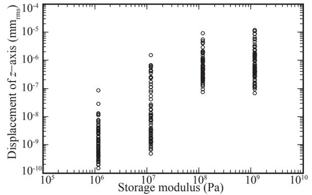
**Fig. 2** Relationship between displacement of  $z$ -axis at top of the surface layer and the storage modulus.
