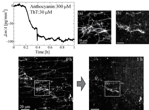
Fig. 2 The time course of mass per unit area on the surface measured by WE-QCM and fluorescence images at same point by TIRFM in dissociation process as flowing poly-phenol anthocyanins solution.
