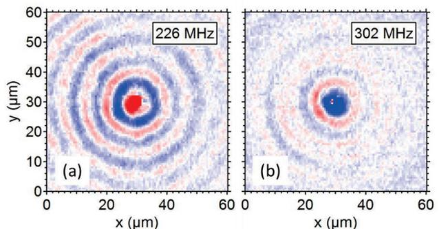
Fig. 2 Experimental images of acoustic surface waves on the microsphere metamaterial at (a) 226 MHz and (b) 302 MHz, probed from the back side.
