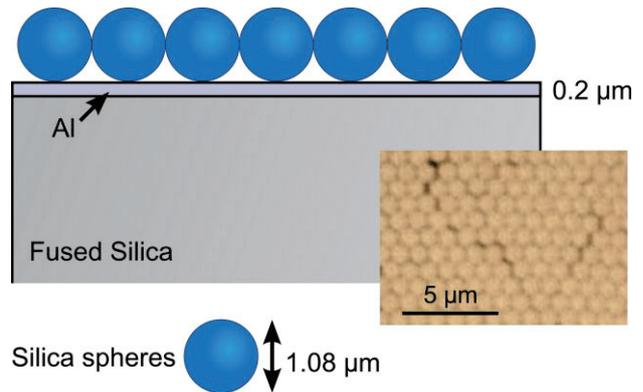
Fig. 1 Cross-sectional diagram of the metamaterial sample structure. Inset: Optical image of the sample surface
