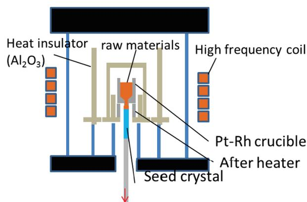
Fig. 1 Pattern diagram of  $\mu$ -PD method
