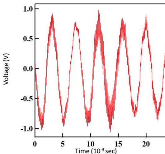
Fig. 3 Time vs. voltage diagram of CNGS crystal generate with the sound from speaker.
