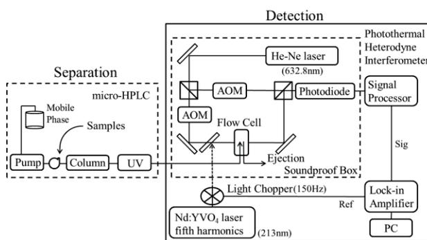
Figure1. Device configuration of PHI combined with micro-HPLC
