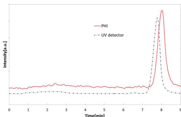
Figure2. Chromatogram of PHI and UV detector
