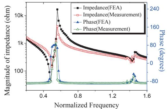
Fig. 3 Comparison of the modeled and measured impedance spectra of the Tonpilz transducer in air.
