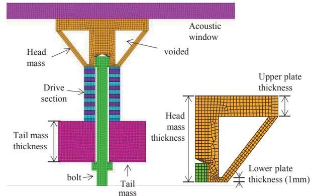
Fig. 1 Schematic structure of the Tonpilz transducer with the void head mass.
