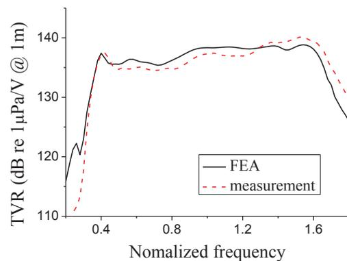
Fig. 5 Comparison of measured and modeled TVR spectra in water.
