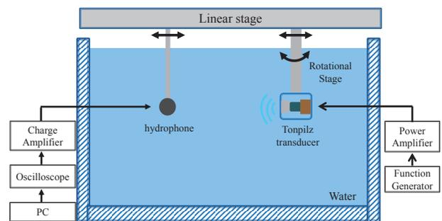
Fig. 4 Schematic diagram to measure the TVR of the Tonpilz transducer prototype.
