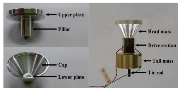
Fig. 2 Photograph of the Tonpilz transducer prototype with the void head mass.
